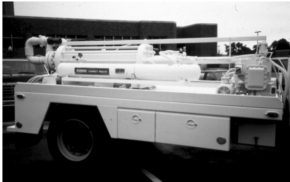
Figure 14-6 Typical small-volume prover.
