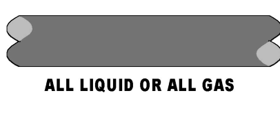
Figure 6-2 Single-phase flow is required.
